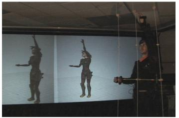
Testing the accuracy of two motion capture suits simultaneously
