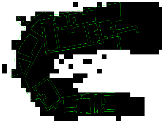
Figure 4: The sun position was calculated using the altitude and azimuth for Sept 21, 3200 B.C.E, at 2:00 pm. A ray was cast from the center of each ground square to the sun. If no objects (walls or roof) intersected the ray, the square was in sunlight and is shown in white; otherwise, the square was in shade and is shown in black.
